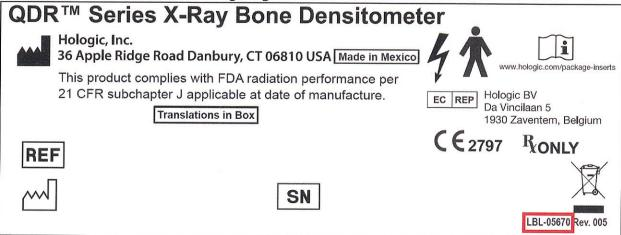
3. "REF" indicates the Horizon Model and "SN" is the identification Serial Number of the system. "" indicates the date of manufacture of the system.
